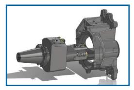
CAT 50 Special Combination Boring Tool designed using sophisticated in house Rigibore design software.
