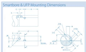
No machine spindle modification required. Smartbore bars can be carried in a standard magazine and tool management system.
